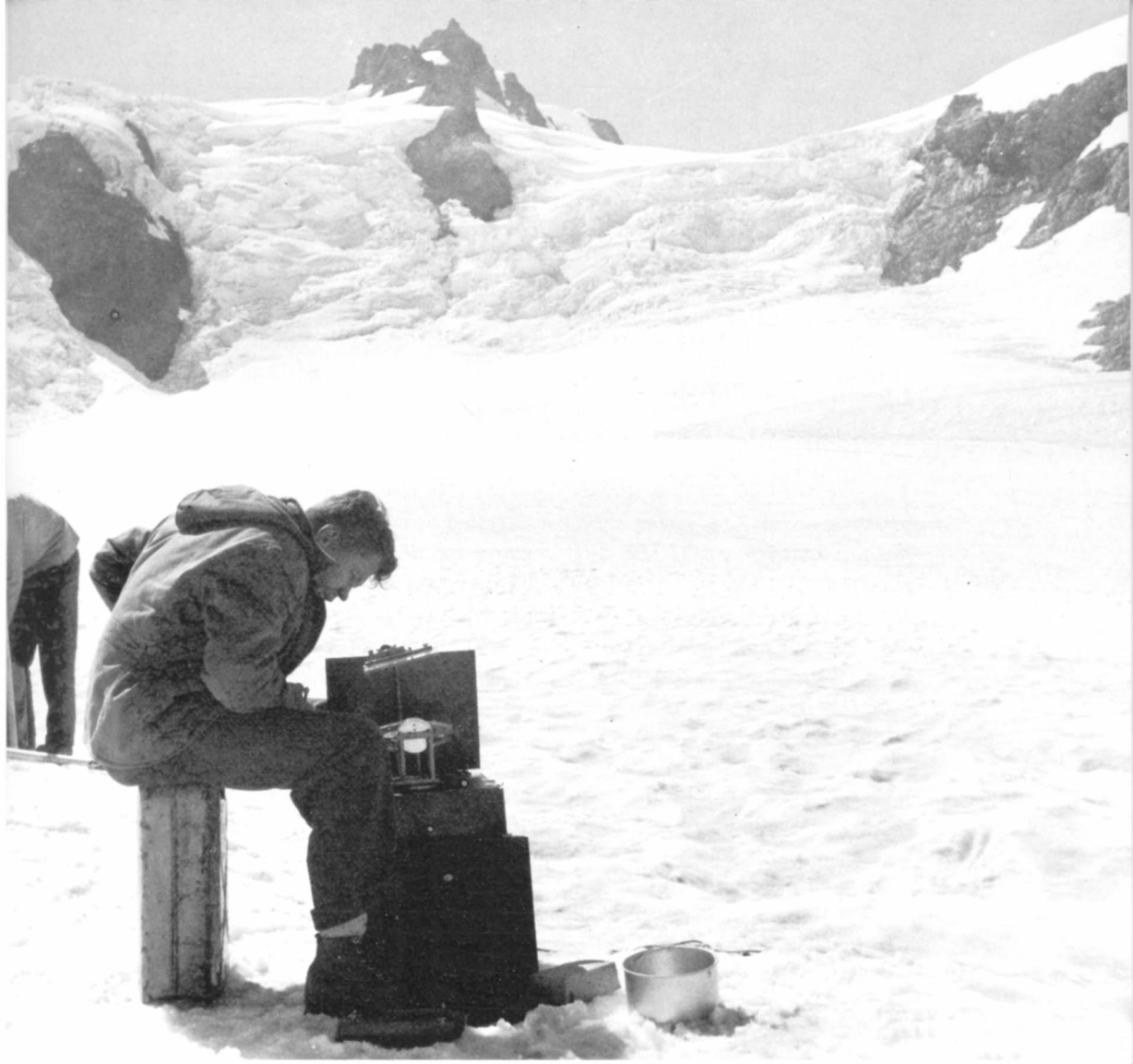
A —Looking southwestward up the Blue Glacier in the Olympic Mountains, Washington, to the 1000-foot icefall. Universal stage for measurement of ice crystal orientation in the foreground. August, 1957.
