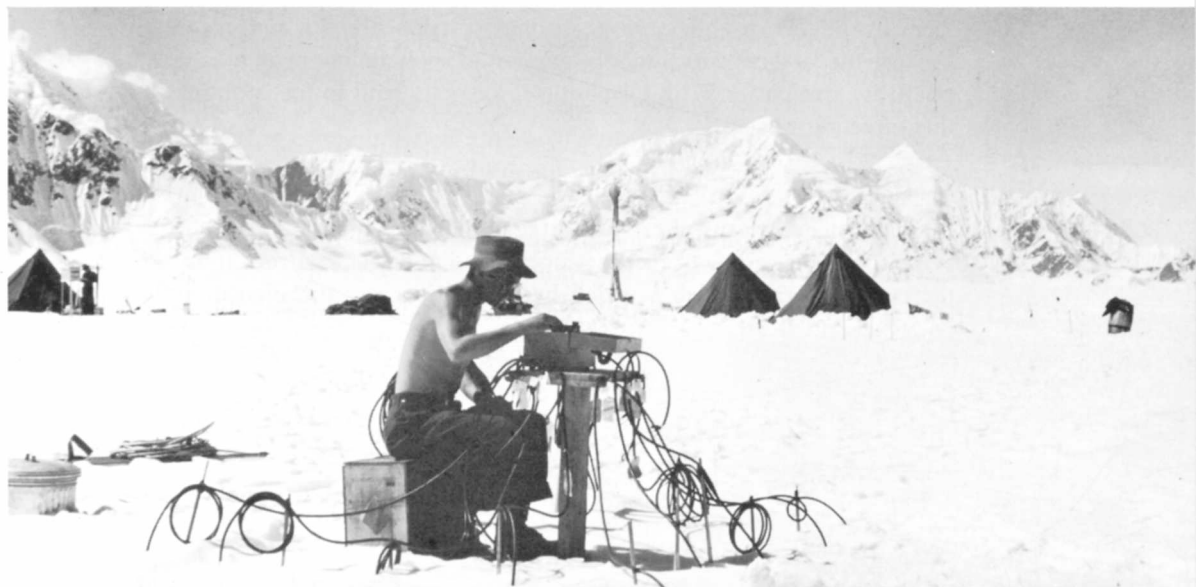
B —Measuring the warming up of the winter's chilled layer on a temperate glacier, upper Seward Glacier, Alaska, June, 1949.
