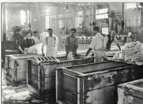
Interior of a dye house. Skeins of silk thread were dipped in the vats of hot water and chemicals.
