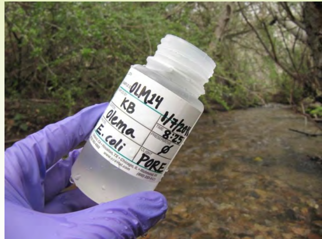
An autoclavable bottle used to sample bacteria in Olema Creek. Photo by Katie Booth
