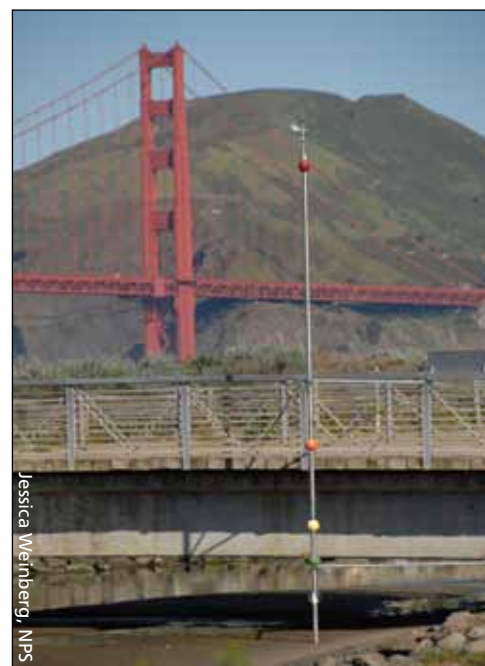
Brightly colored balls show how high the water will get at Crissy Field under different sea level rise scenarios
