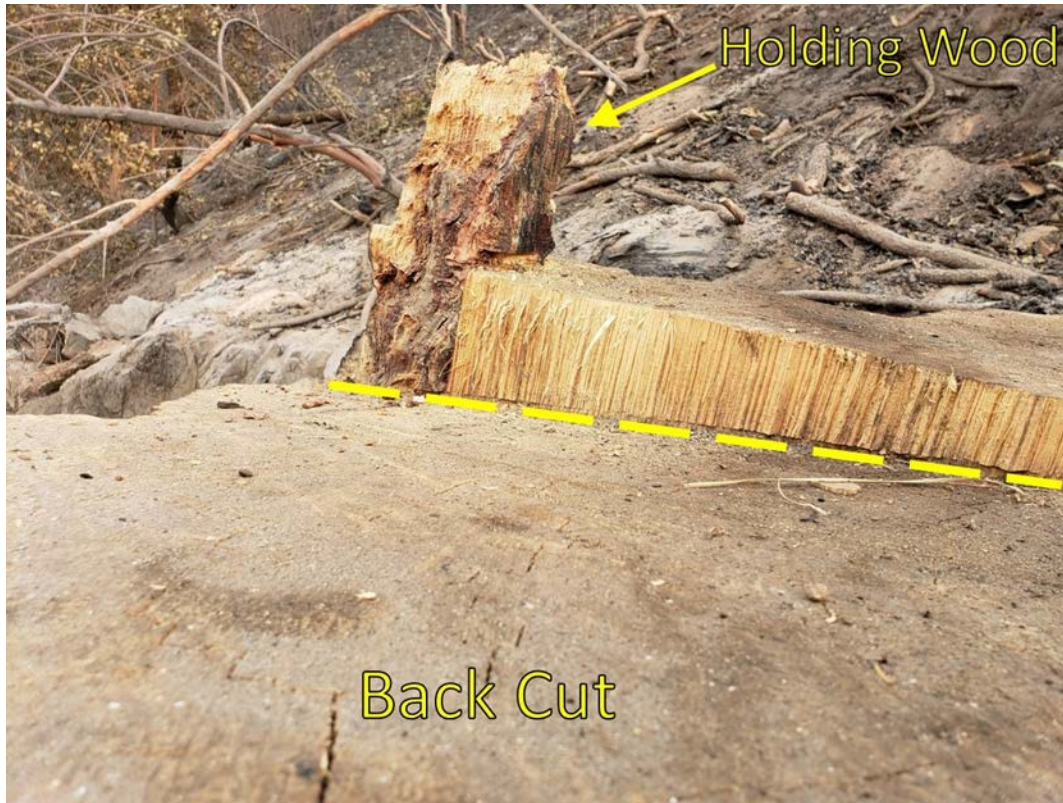
Figure 14: View of stump showing surface planes for the face and back cuts. Dashed line indicates the height difference between cuts on the offside.
