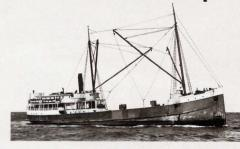
The 1915 steam schooner Wapama (above) is undergoing thorough preservation treatment at a temporary berth at the Bay Model Visitor Center in Sausalito. Steam schooners like Wapama carried both cargo and passengers, gradually replacing old sailing schooners like C.A. Thayer. These wood-hulled steamers were designed for the Pacific Coast trade, carrying lumber south and general cargo north.
