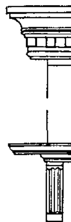
CORNICE AND SILL OF THIRD FLOOR WINDOWS OF MAJOR SOUTH GABLE
