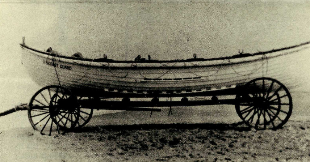
Self-bailing surfboat on boat wagon — note scuppers and hand rails.
