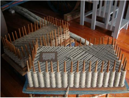
Faking rig for rope used with a Lyle gun
