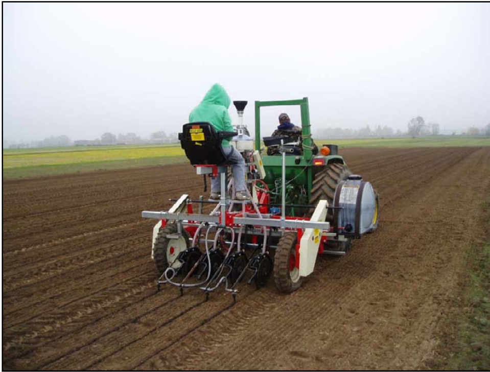
The Corvallis PMC's new precision cone-seeder equipped with a carbon-banding unit.
