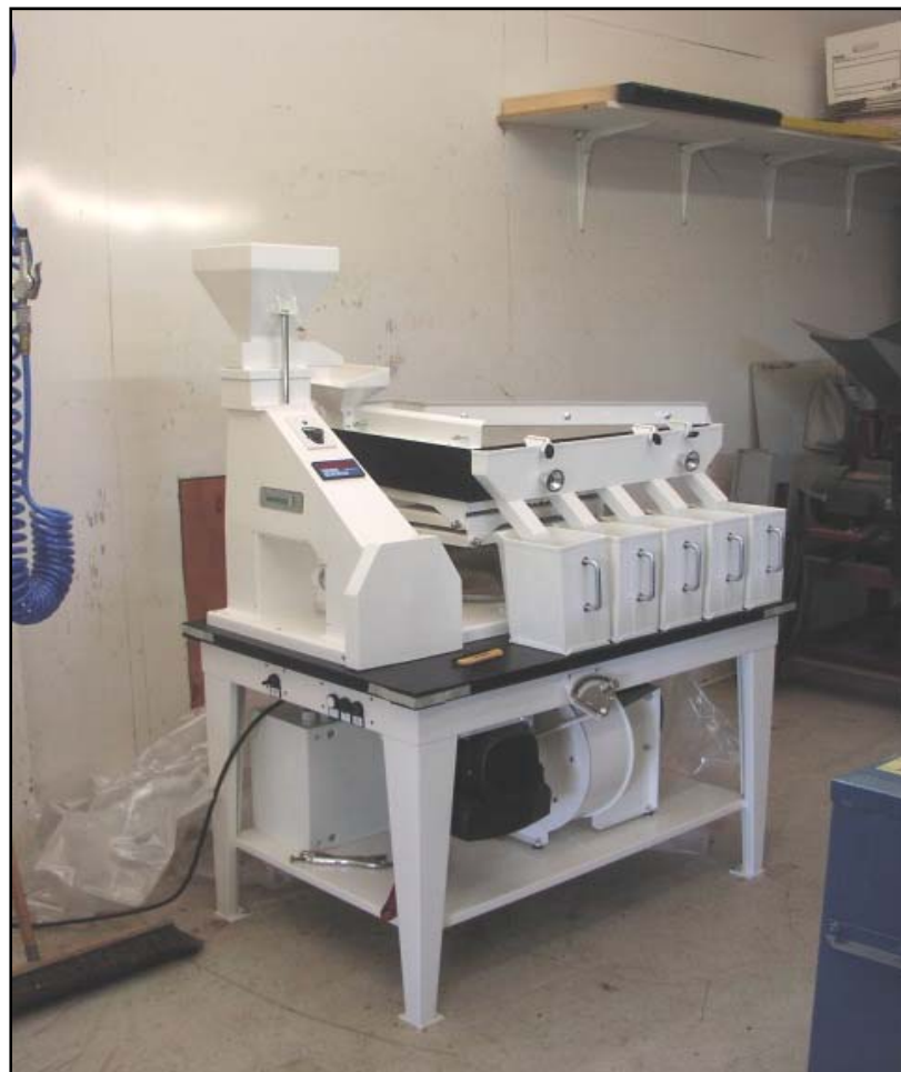
A lab-sized gravity table was added to the PMC's seed cleaning facilities this year.
