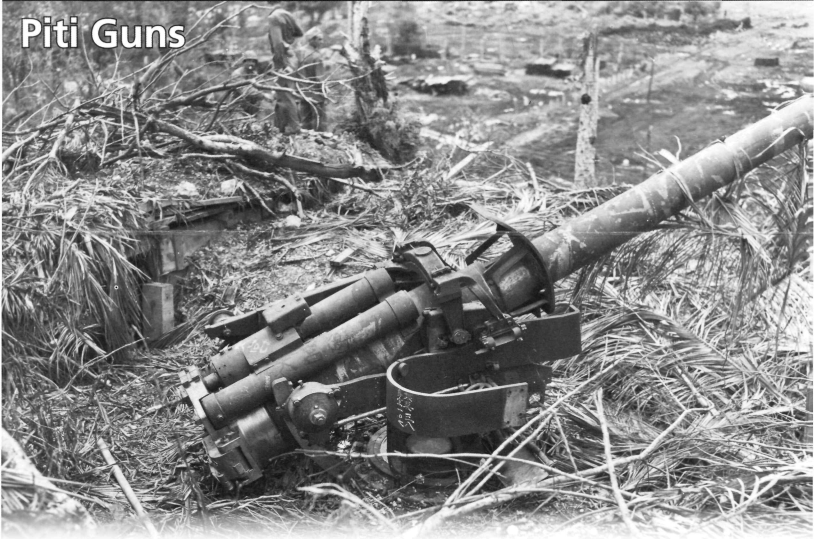
October 5, 1944: A Japanese Vickers-type Model 3 (1914) 140-mm (5.5 inch) coastal defense gun stands intact over the ruins of Piti.
