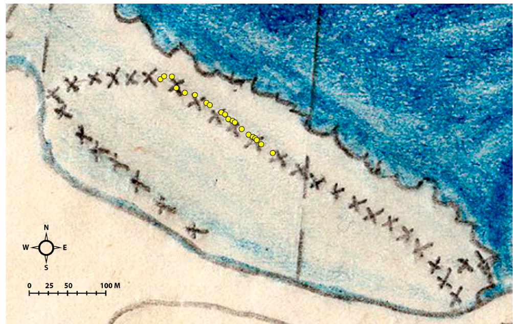
Figure 7. Map showing location of blast craters (yellow circles) in reef flat within the Asan Beach Unit, documented using GNSS RTK as part of this project, overlaid onto a hand-drawn historic map by UDT 3. Image: Nicole LaRoche, NPS.
