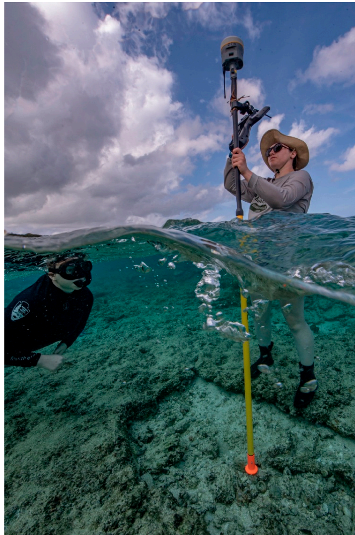
Figure 6. Project team members documenting the location of a blast crater within the Asan Beach Unit using GNSS equipment. Image: Brett Seymour, NPS.
