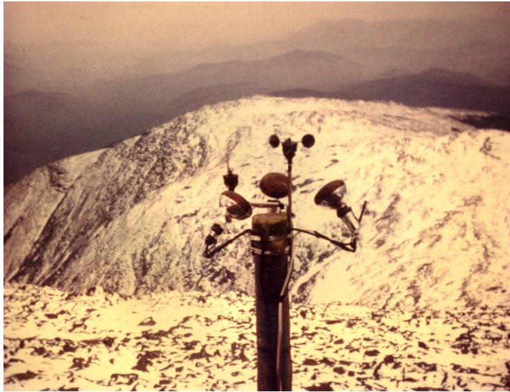
Prototype infrared anemometer test array, SE side of TV Building. The site overlooks Tuckerman's Ravine. After D. E. Glidden, 1972-73.
